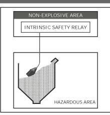
ATEX The 🐼 proof devices ATEX certified are now compulsory in the majority of silos. They allow in total security the stopping of the silos' filling and the installation of high level "Alarms" as a complement of other detection systems. They are inexpensive and easy to install.
